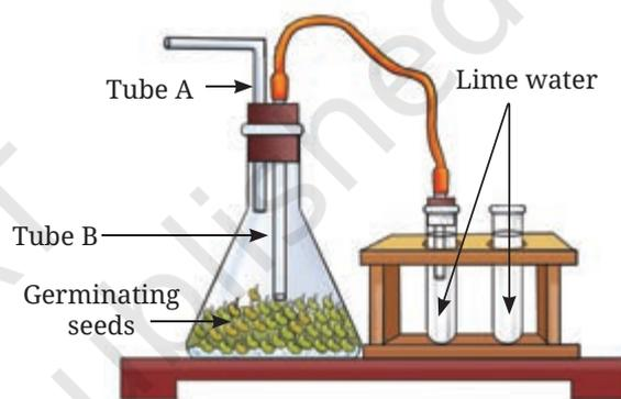
Fig. 10.9: Set-up to test respiration in plants
